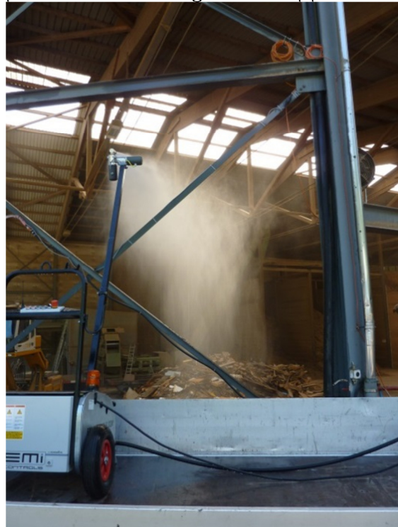
The L3 Fogging Lance used to reach a dusty pile indoors, accessing through supports.
