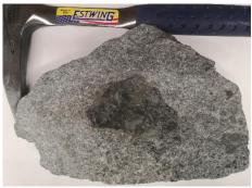
Image: Hand specimen of fresh Diorite Porphyry showing black xenoliths.
